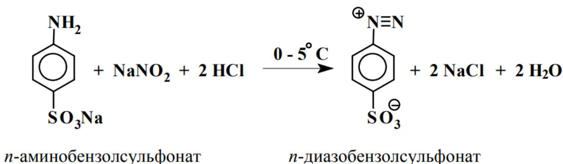
Preparation of *p*-diazobenzenesulfonate\*. Dissolve 2.3 g of sodium sulfanilate in 5 ml of water in a beaker and add to it a solution of 0.7 g of sodium nitrite ( $\text{NaNO}_2$ ) in 10 ml of water (Note 1). While cooling with ice or snow and stirring, the resulting solution is poured into 10 ml of 4 N hydrochloric acid solution. Not earlier than 5 minutes after draining the solutions, a sample of the reaction mixture
