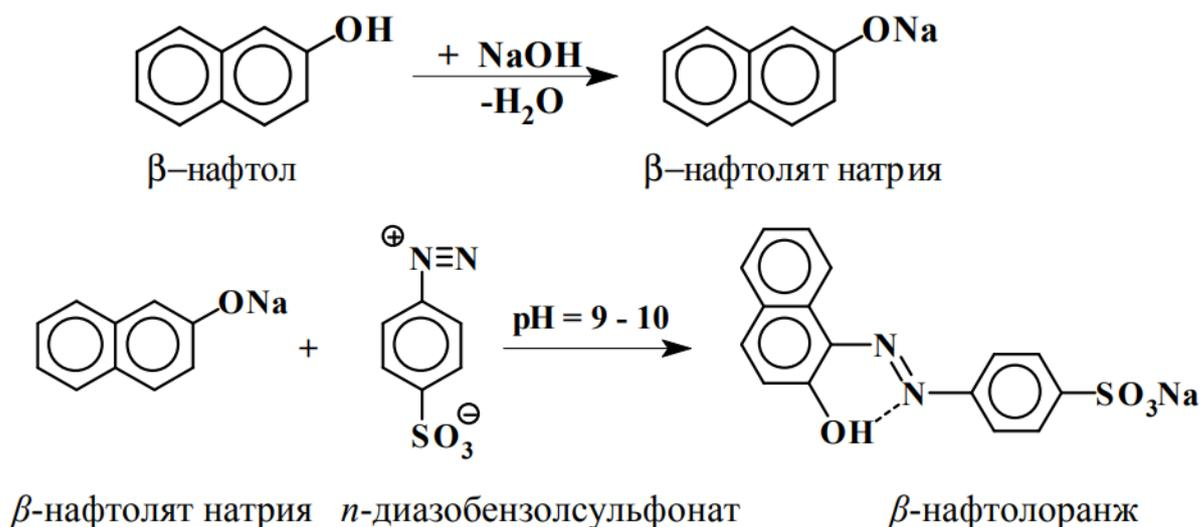
Dissolve 1.4 g of finely ground  $\beta$ -naphthol in 20 ml of 2 N sodium hydroxide solution with gentle heating. A solution of sodium naphtholate is cooled in a mixture of water with ice or snow, and a cooled suspension of p-diazobenzenesulfonate is added to it. After some time, the crystallization of orange-yellow leaves of the sodium salt of the dye begins. To reduce the solubility of  $\beta$ -naphthol-orange, 3 g of
